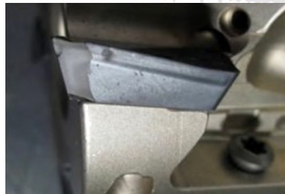
Figure 1. Tool wear observed on a high-performance machining center after 38 roughing passes in 4140 alloy steel. Replenish cost was $60 for four new inserts.
