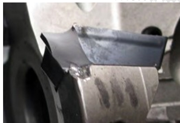
Figure 2. Tool wear observed on a conventional machining center after 28 roughing passes in 4140 alloy steel. Replenish cost was $924 for four new inserts and a tool body replacement.
